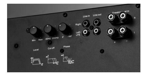
• A: Volume – Controls subwoofer level. **This amplifier has a very high** gain. Set the level @ 10 - 11 o'clock or lower. Using at settings greater than 12 o'clock could cause failure.
