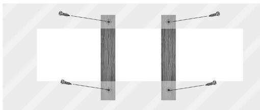
**VERY IMPORTANT:** When mounting the wood supports behind the drywall keep the screws as close as possible to the cutout opening. No more than 7/16" away from the opening or the 1/2" collar that goes around the soundbar will not cover over the screw heads.
