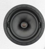
The CI-IC8 is our top-of-the-line solution for music reproduction and height channel applications. Consisting of an 8" Kevlar driver, 1" Tetoron pivoting tweeter, high-grade crossover, and mid/high-frequency acoustic switches, this speaker is the ultimate performer.
