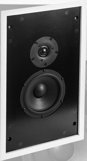
The CI-IW6 and CI-IW8 are 6" and 8" respectively two-way compact sized in-wall loudspeaker systems capable of extremely high sound pressure levels, while maintaining true sonic fidelity. Their 3/4" thick front panel and high acceleration carbon/wool woofer provide dynamics and clarity associated with in-wall systems costing far more. A highly regarded 1" Vifa™ DX dome tweeter, combined with a two-pole high transfer crossover, produces a wide power bandwidth and "fill".
